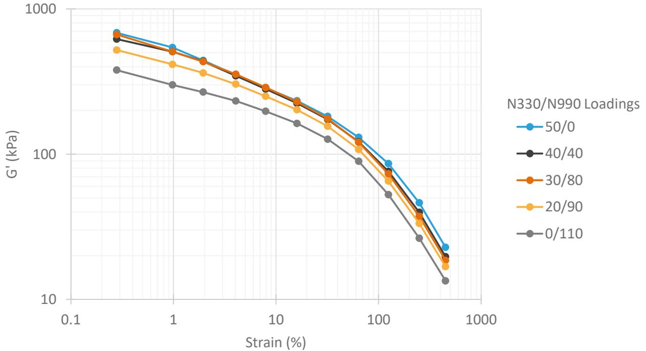
**Figure 5.** Storage modulus as a function of strain amplitude at a temperature of 60°C and frequency of 0.63 rad/s. Significant reduction in modulus as N990 replaced N330.
