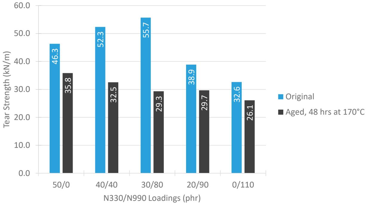
**Figure 11.** Die C tear strength, original and air oven aged 48 hours at 170°C, for each compound. Aged tear strength decreased as N990 loading was increased.
