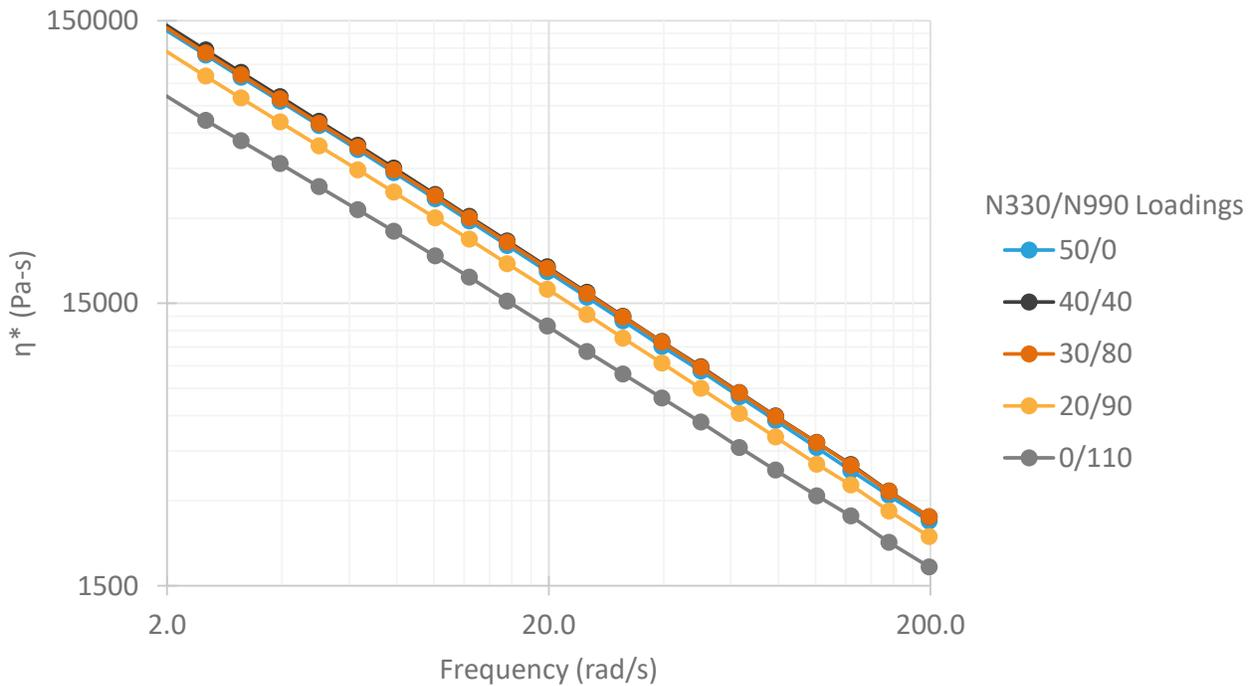
**Figure 4.** Complex dynamic viscosity as a function of frequency at a temperature of 100°C and strain amplitude of 7.0%. The viscosity decreased significantly as N990 replaced N330.
