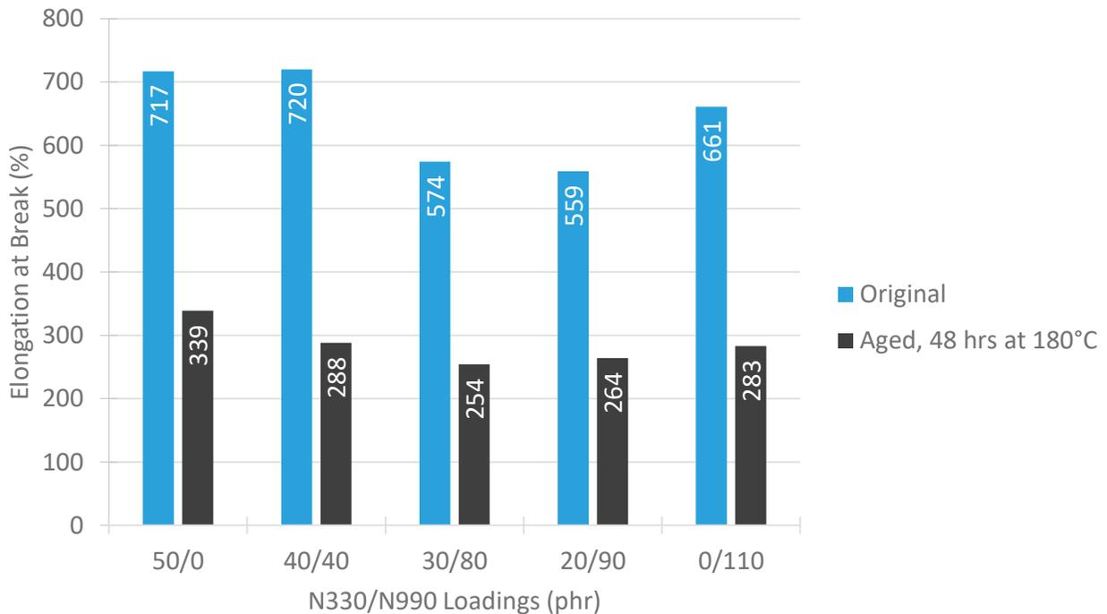
**Figure 10.** Elongation at break, original and air oven aged 48 hours at 180°C, for each compound. No clear trend in elongation was observed.
