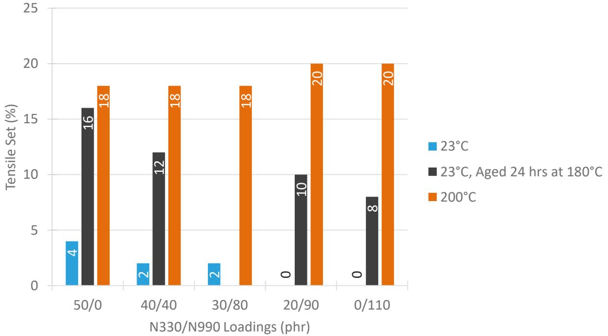
**Figure 13.** Tensile set, original at room temperature and 200°C and air oven aged 24 hours at 180°C at room temperature, for each compound. Room temperature tensile set decreased with increased N990 loading. High temperature tensile set showed no significant change.
