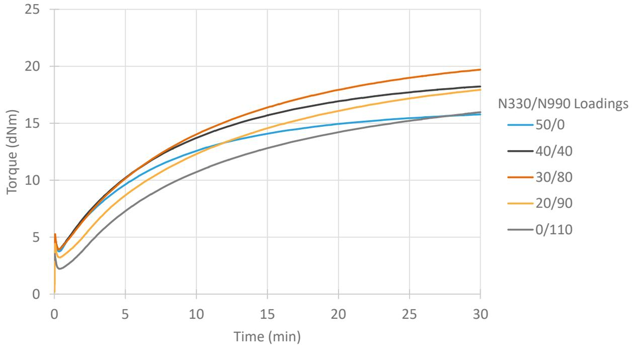
**Figure 3.** MDR cure curves at 190°C and 1° arc. Marching modulus was evident. A slight increase in scorch times at high loadings of N990 was observed.
