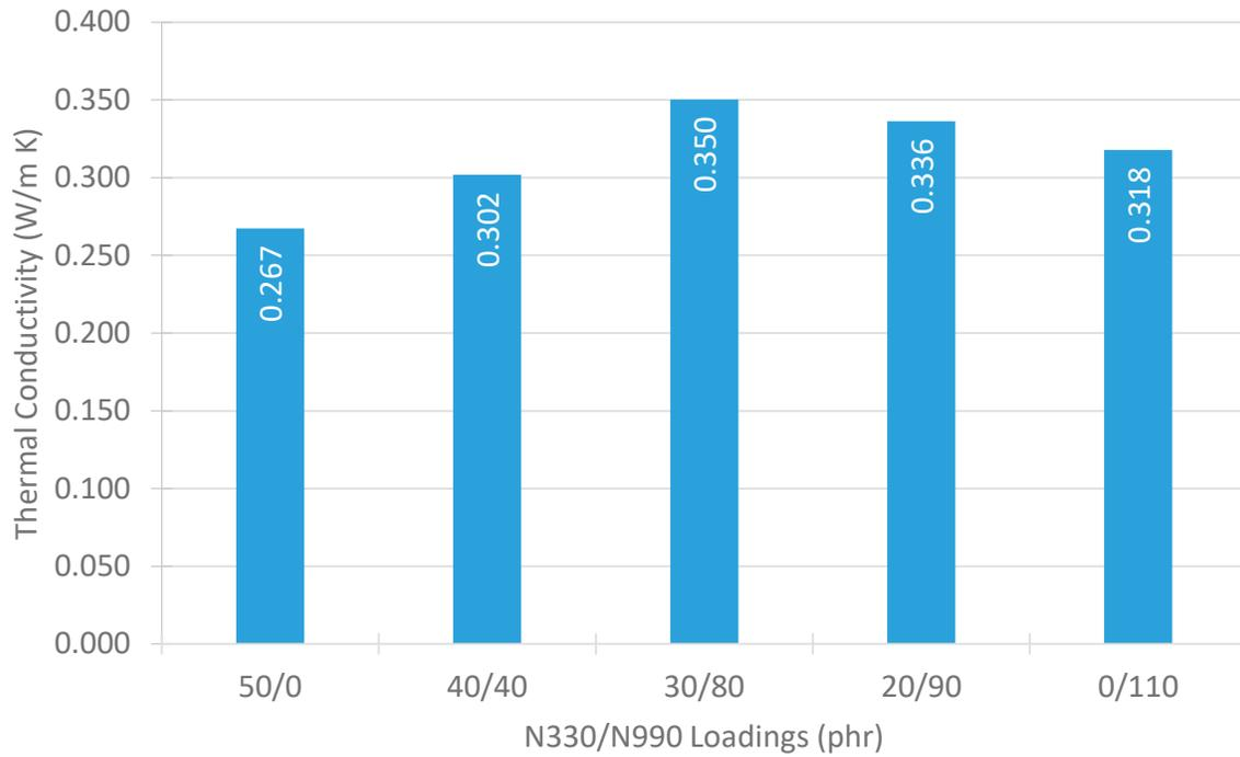
**Figure 15.** Thermal conductivity for each compound. Higher thermal conductivity was observed for the compounds with N990 compared to the control compound.
