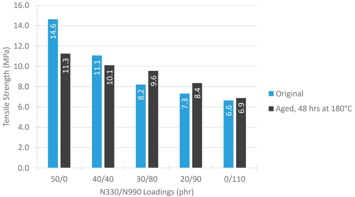
**Figure 9.** Tensile strength, original and air oven aged 48 hours at 180°C, for each compound. Tensile strength decreased as N990 loading was increased.
