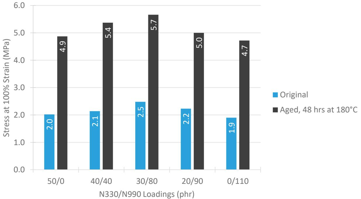
**Figure 7.** Stress at 100% strain, original and air oven aged 48 hours at 180°C, for each compound.
