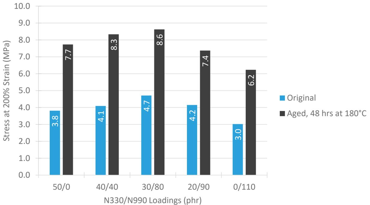
**Figure 8.** Stress at 200% strain, original and air oven aged 48 hours at 180°C, for each compound.
