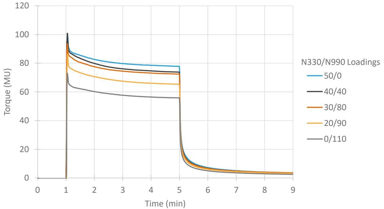
**Figure 1.** Mooney viscosity at a temperature of 100°C. Viscosity dropped considerably as N330 was replaced with N990.
