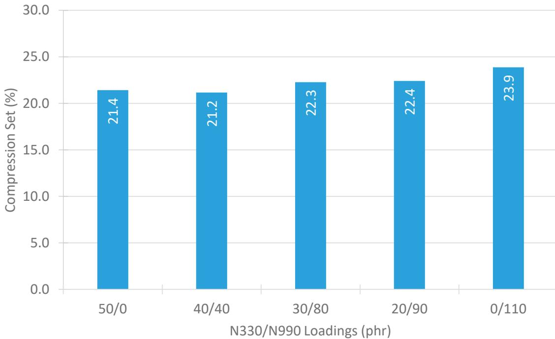
**Figure 14.** Compression set after 70 hours at 100°C for each compound. No significant change was observed.
