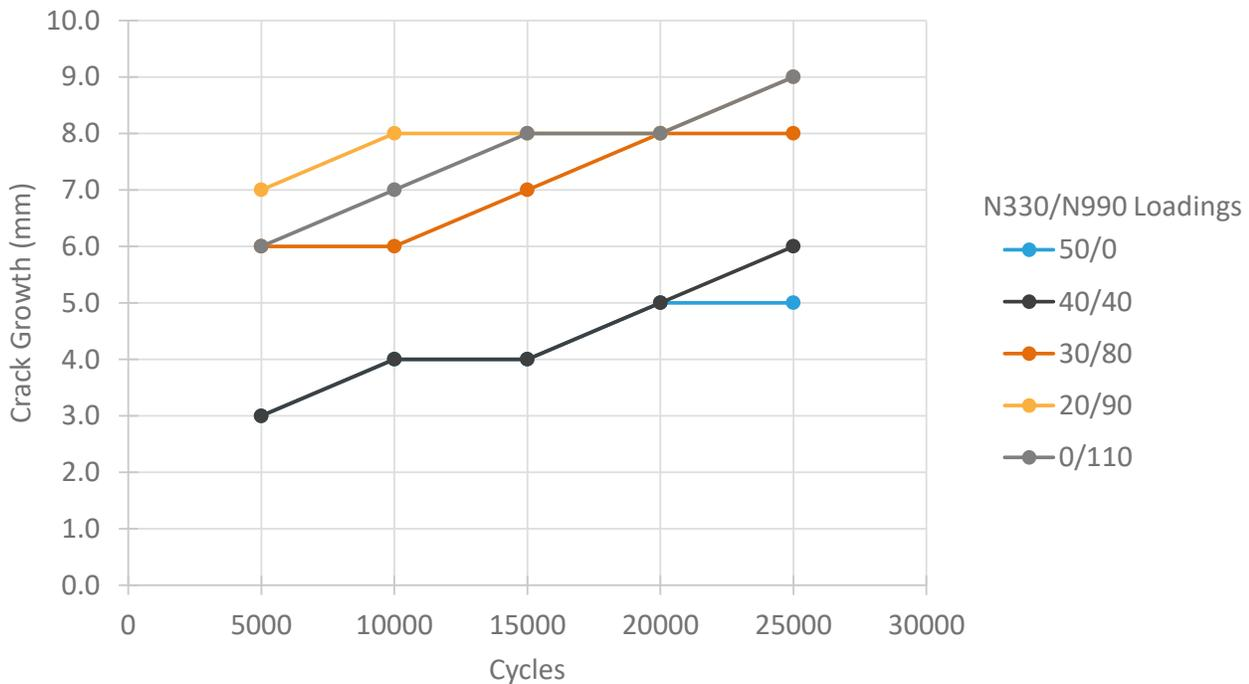
**Figure 12.** DeMattia crack growth for each compound. Crack growth increased when N990 loading was increased to 80 phr. There was no change in crack growth at N990 loading of 40 phr.
