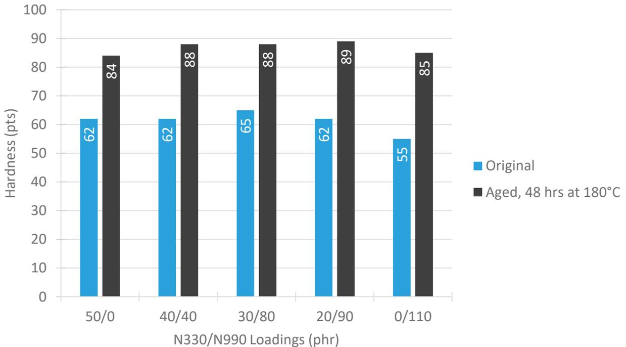
**Figure 6.** Hardness, original and air oven aged 48 hours at 180°C, for each compound. All compounds met the 60±5 durometer specification. There was no significant difference in aged hardness.
