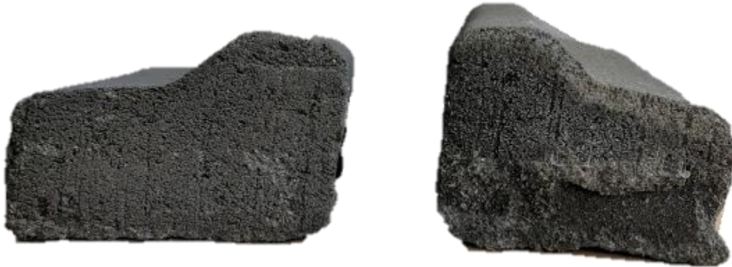
Figure 2. Untouched (left) and weathered (right) samples of Carbocolor in concrete.
