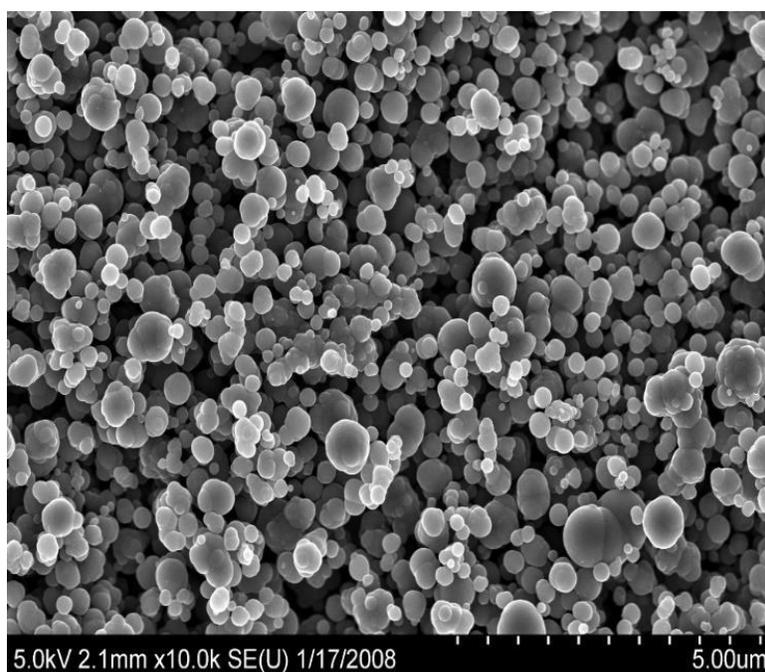
**Figure 1.** SEM image of Thermax<sup>®</sup> N990
