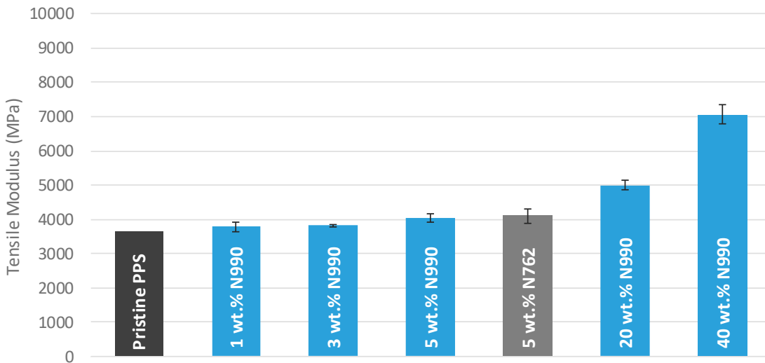
Figure 2. Tensile modulus of PPS composites. Tensile modulus increased with filler loading.
