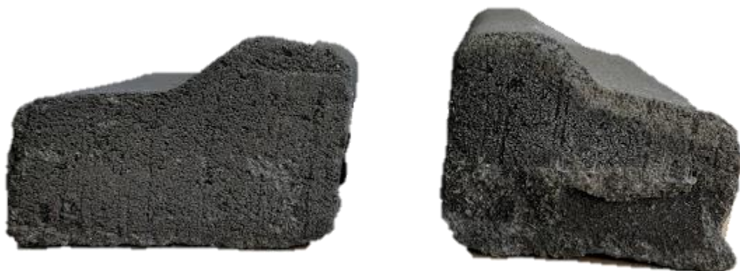
Figure 1. Untouched (left) and weathered (right) samples of Carbocolor pigment in concrete
