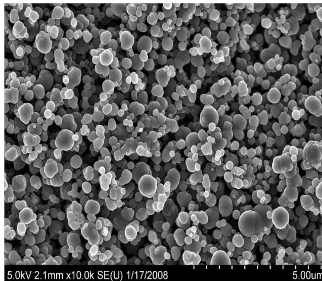
Figure 1. SEM imaging of N990/N991 Thermax<sup>®</sup> Ultra Pure showing spherical particle shape and approximate particle size
