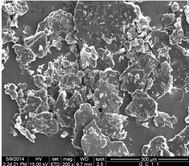
**Figure 2. SEM imaging of graphite demonstrating particle shape**
